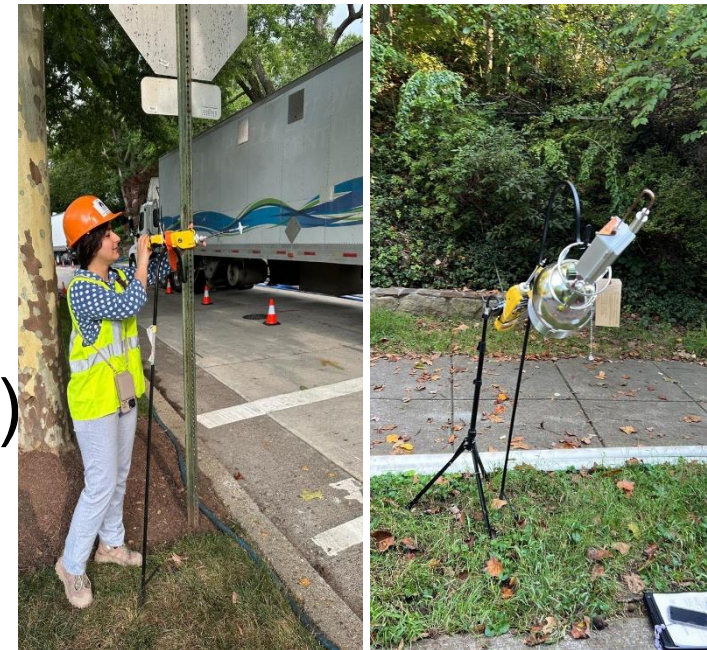
Continuous TVOC Measurement Using PID Positioned Upwind and Downwind of the Insertion Manhole
