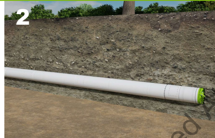
2 Soil excavation with AVNS & pipe jacking process
