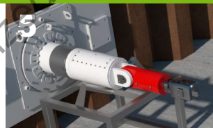
2 Soil excavation with AVNS & pipe jacking process
