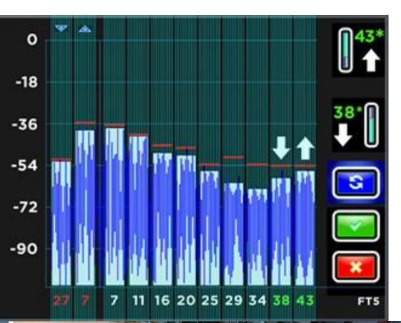
**Frequencies** (sub-kHz, 7.5-45 kHz) Go low for passive, high for active
