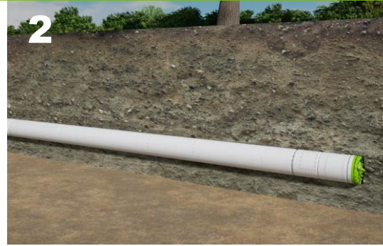
2 Soil excavation with AVNS & pipe jacking process
