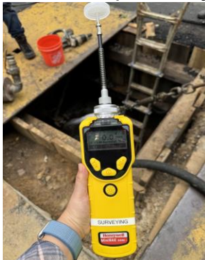
TVOC Measurement Using Hand-held PID
