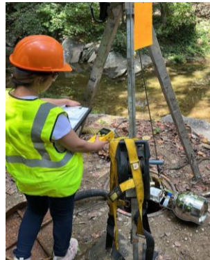
TVOC Measurement Using Hand-held PID
