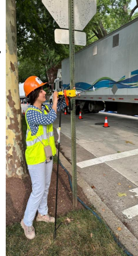
Continuous TVOC Measurement Using PID Positioned Upwind and Downwind of the Insertion Manhole
