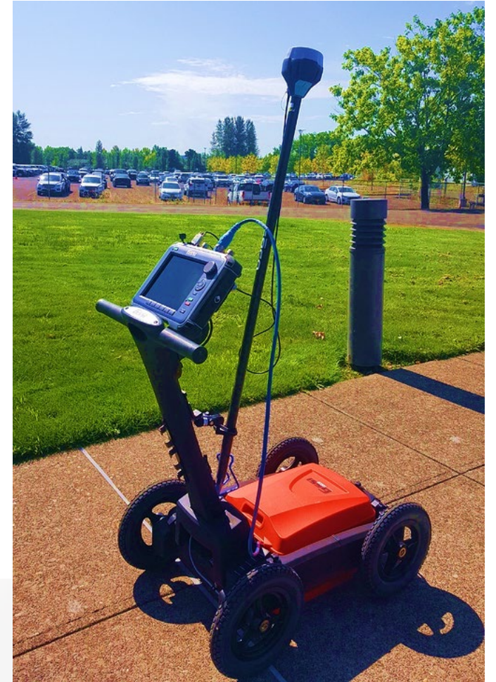
Hyper Stacking GPR Survey Unit
