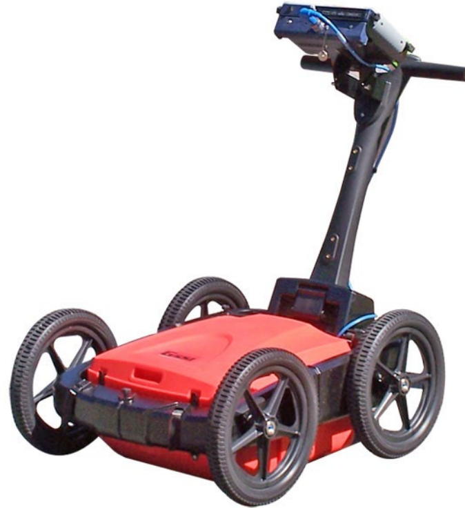
Hyper Stacking GPR Survey Unit
