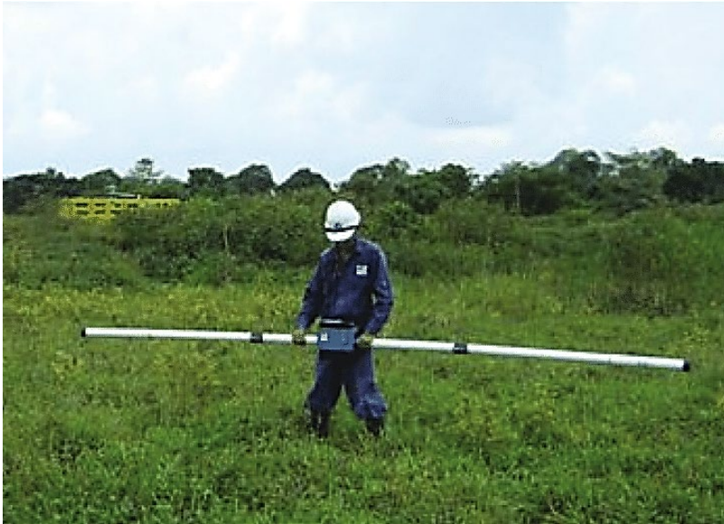
EM31-MK2 Ground Conductivity meter
