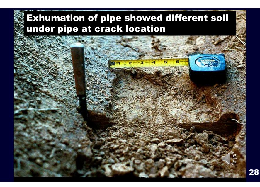
Note different rate of drying. Pipe was rested on soil mounds used for grade, soil not compacted under pipe. Over time, mounds became hard spots
