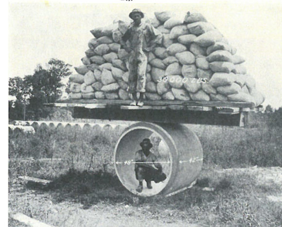
48-inch diameter pipe, 3½ feet long, at Columbia, S. C., loaded to 30,000 pounds with knife-edge loading. No crack shown in the pipe.
