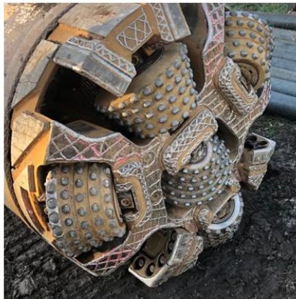
Cutters after 140m of tunnelling
