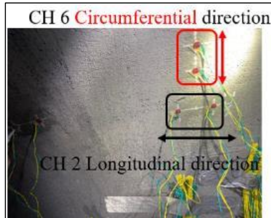
Full-bridge (thermally compensated) gages for circumferential and longitudinal strain
