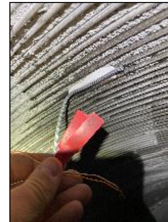
Polyimide substrate gage (quarter bridge) on wire
