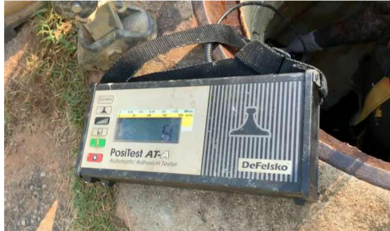
19 Year Reinspection Adhesion pull test of a DeKalb County manhole
