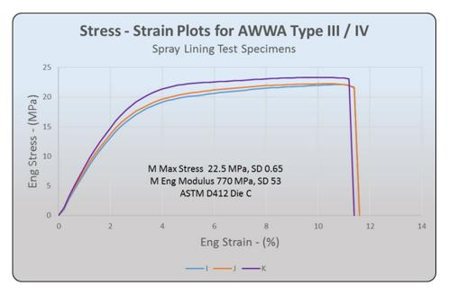
The solution requires a product with a modulus of 450,000 (structural portion of the composite) with a specific elongation of 5%, combined with a more elastomeric product with a modulus of 150,000 and a specific elongation of 400%. This combination is ideal for SIPP. Total liner design including its thickness is an engineered solution that we develop through information provided by the EOR for each project.
