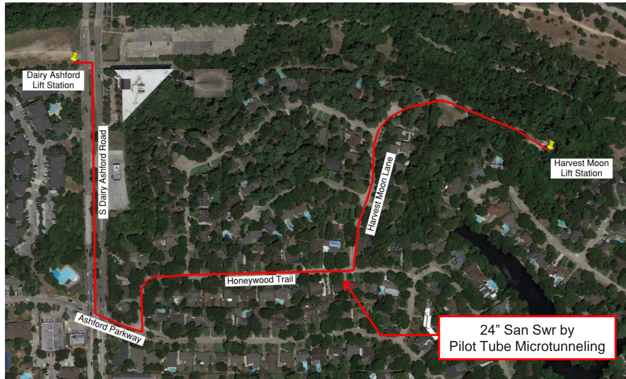
Proposed Sanitary Sewer Alignment
