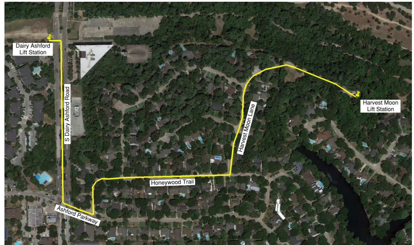
Parallel Sanitary Sewer and Force Main Alignment
