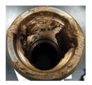
Proper Thread Compound coverage for Rotary Shouldered Connections
