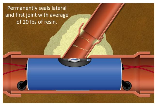
Applicable for both lined and un-lined main pipe.
