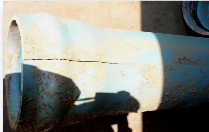
Slow Crack Growth & Rapid Propagation
