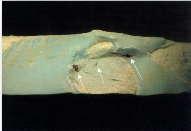
Small Defects => Crack Initiation
