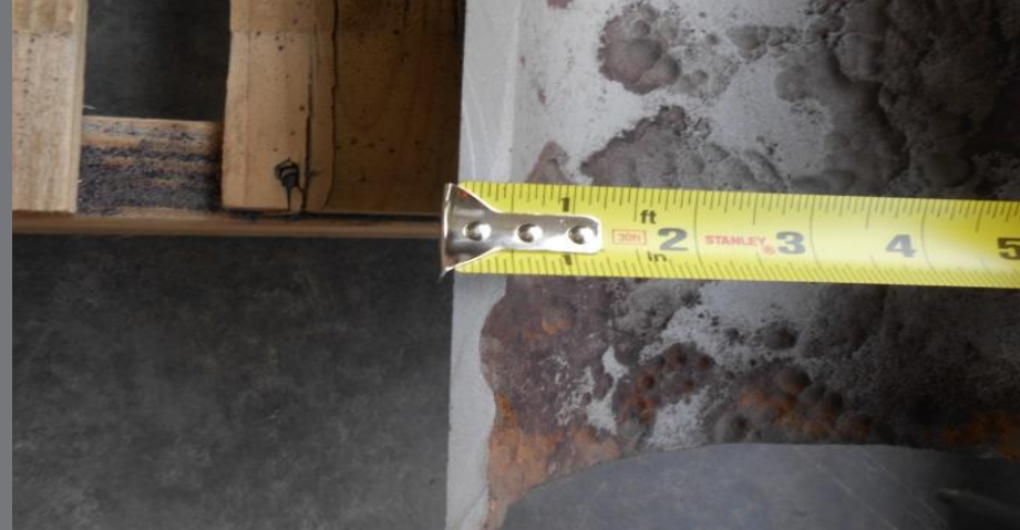
Uncorroded pipe measurements were generally 7/16-inch thickness (0.43 inch).
