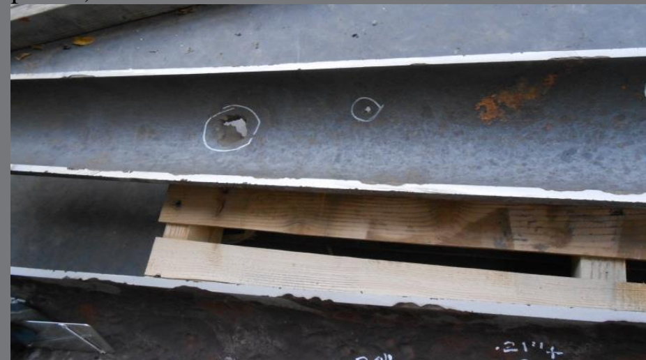
Seven pipe segments were split longitudinally into 14 pieces, then sandblasted.
