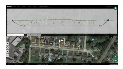
Create a bore designed to avoid utilities and be more productive  Add your as-drilled data after the bore is complete right from the locator
