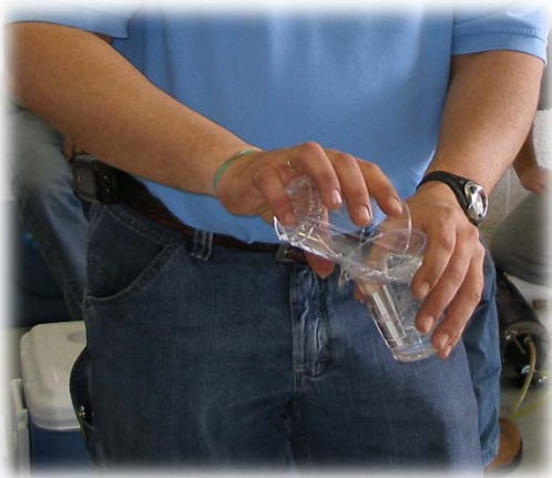
Standard cup test for gel time verification
