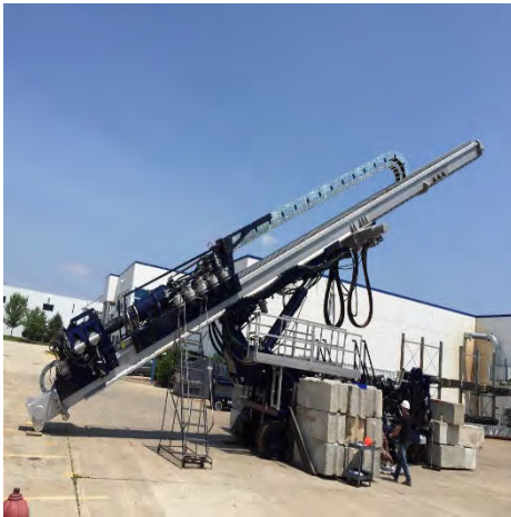
Slant directional drilling, SDD (since 2011)
