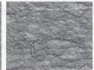
CSP 6 (heavy shotblast)
