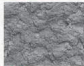
CSP 7 (heavy shotblast)
