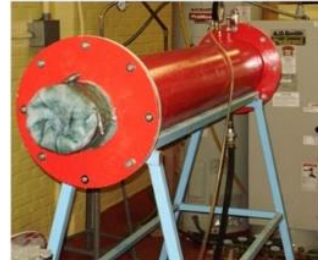
Liner Inversion Chamber
