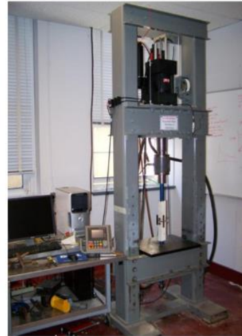
Servo controlled test machine, large, for tensile and flexure testing
