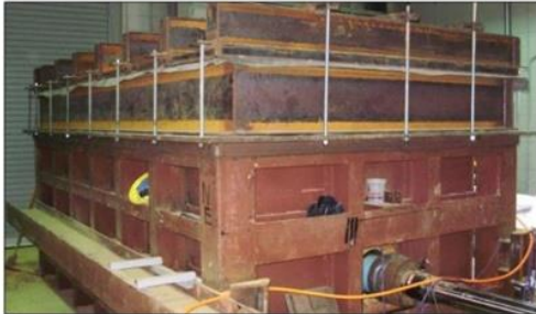
Soil box (small 12'x6'x6', large 10'x20'x11')
